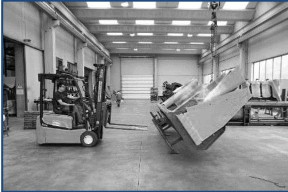
Avoid or limit any sliding of the header, controlling its movement with the tips of the forks.
