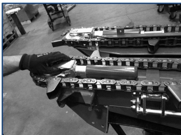
Remove the chain (in the marked phase)
