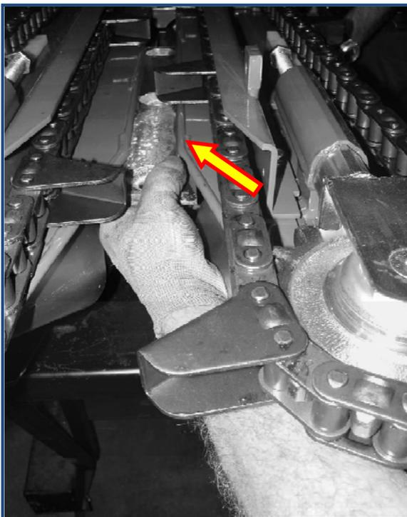
Adjust the cob snapping blades so that you can pass through with the Sunflower Kit
