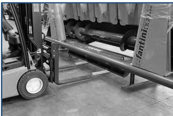
Use the tips of the forks of the forklift truck to fold the header, lifting it from one side.
