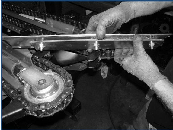
Secure the two sheet metals without tightening the screws so as to leave a gap between them
