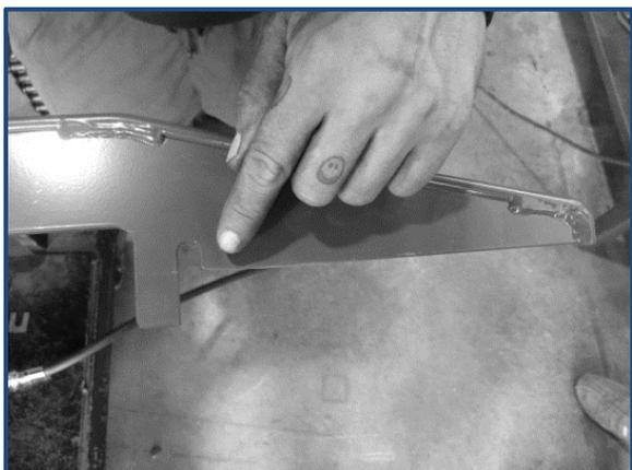
If necessary, cut the right cob snapping blade as shown in the picture
