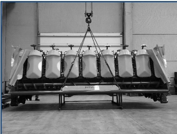
The corn header can be equipped with an iron support for transport in the vertical position.
