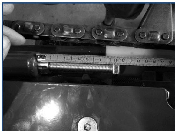
Tighten the pusher up to a measure of 115 mm, see picture.
