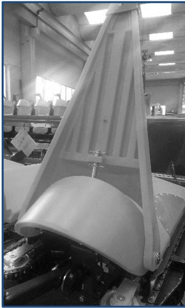
**Transport position.** Use the pipe supplied as standard equipment to block rotation of the plastic point
