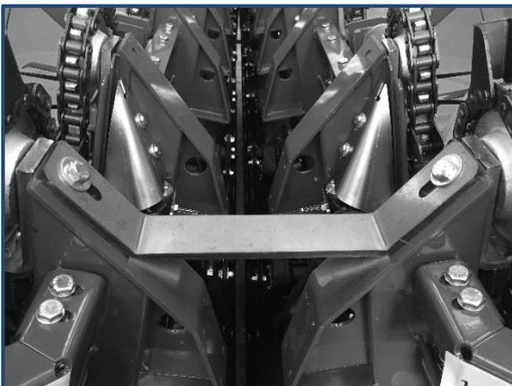
The folding version can be supplied with plates, bars or other supports to facilitate the transport.
