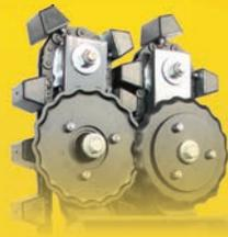
Two counter-rotating **Cutting Discs** gently cut the sunflower stalk without shaking, resulting in minimal seed loss.
