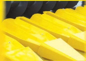
**Specially Shaped Collecting Pans** are designed to catch anything falling from the sunflower head. They are tilted backwards ensuring everything falling on them flows easily to the auger, thereby minimizing seed loss.
