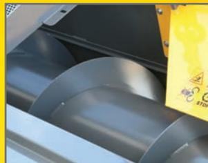
The **High Capacity Auger** ensures a constant crop flow to the combine feeder house.
