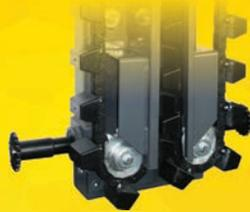
The **Row Units** are connected by double chain couplers and telescoping shafts, which can be removed quickly for reduced downtime during repairs.
