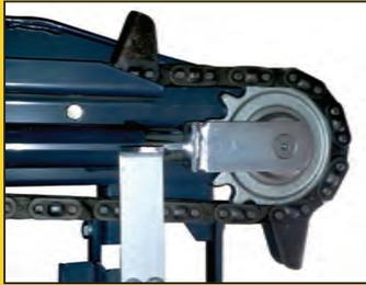
An easily adjustable **Gathering Chain Front Sprocket** ensures optimal reliability in all working conditions.
